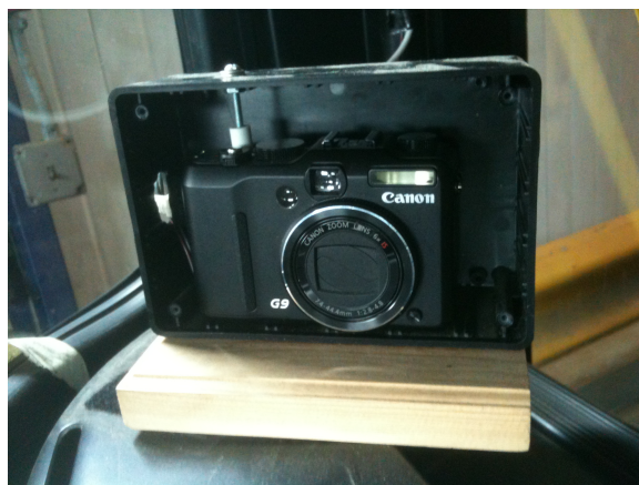
Figure 1: Canon G9 camera mounted inside a bus. The lid of the protecting box is taken out in this picture. The power button of the camera is always pressed down. When the vehicle starts, the bricks turns on instrumenting the camera to start the capturing process.
