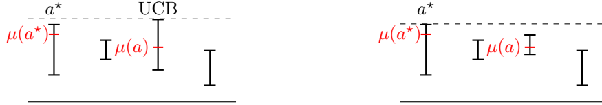
Figure 1: An illustration of the UCB algorithm, showing how every time we play a suboptimal action we acquire information. In the round on the left, arm a is the UCB but it is suboptimal. It will be chosen and the corresponding confidence interval will shrink substantially. In this case the optimal arm a^* becomes the UCB afterwards.
