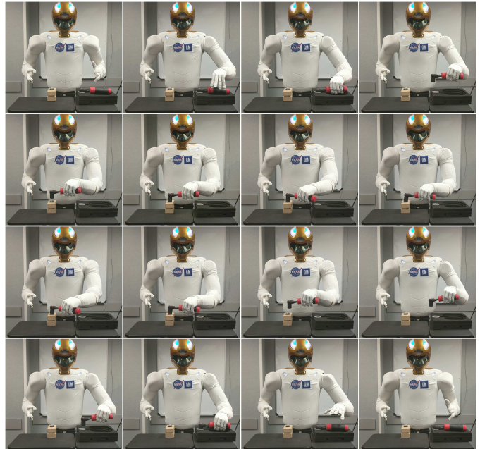
Fig. 9. The ratchet task sequence performed by Robonaut-2. The images from left to right, then top to bottom, show a sequence of actions where Robonaut-2 grasps the ratchet, tightens a bolt on a platform, and puts the ratchet back into a tool holder.
