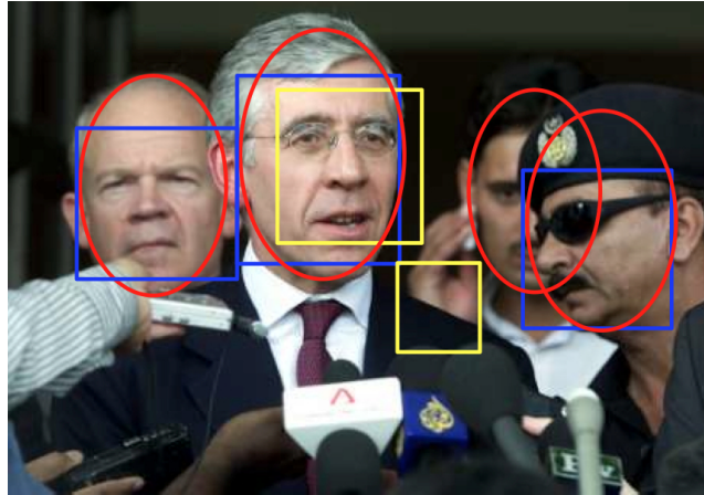
Figure 8. Matching detections and annotations. In this image, the ellipses specify the face annotations and the five rectangles denote a face detector’s output. Note that the second face from left has two detections overlapping with it. We require a valid matching to accept only one of these detections as the true match, and to consider the other detection as a false positive. Also, note that the third face from the left has no detection overlapping with it, so no detection should be matched with this face. The blue rectangles denote the true positives and yellow rectangles denote the false positives in the desired matching.
