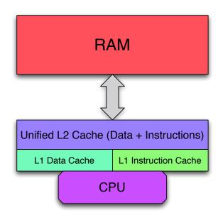
Figure 6.2: Hierarchical cache architecture.
