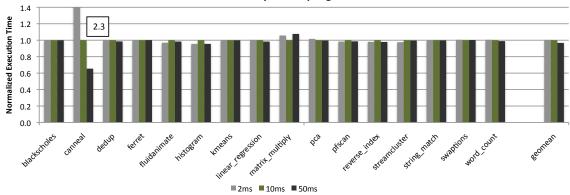
**Figure 9.** SHERIFF-DETECT performance with different sampling rates, normalized to the performance with a sampling interval of 10ms (presented in Figure 7); lower is better.
