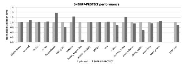
**Figure 8.** SHERIFF-PROTECT performance, normalized to the performance of the pthreads library (see Section 6.4; lower is better). For applications with significant false sharing, SHERIFF-PROTECT can substantially increase performance.
