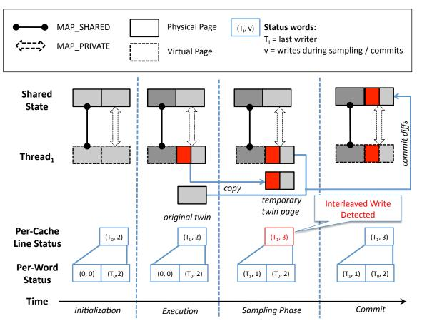
**Figure 3.** Overview of SHERIFF-DETECT's operation. SHERIFF-DETECT extends SHERIFF with page ownership tracking, sampling, and *per-cache line and per-word status* arrays that track frequent false sharing within cache lines. For clarity of exposition, the diagram depicts just one cache line per page and two words per cache line.
