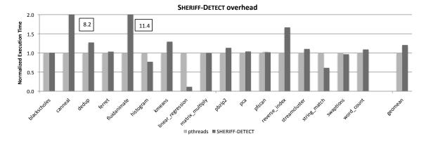
**Figure 7.** SHERIFF-DETECT overhead across two suites of benchmarks, normalized to the performance of the pthreads library (lower is better). With two exceptions, its overhead is quite low (on average, just 20%).
