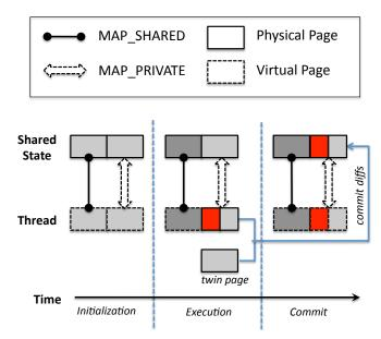
**Figure 2.** SHERIFF replaces pthreads by simulating threads with processes. It exposes an API that enables perthread memory protection and memory isolation on a perpage basis. Each "thread" thus either operates directly on shared memory, or on its own private copy. For the latter, SHERIFF commits diffs to shared mappings at synchronization points (Section 3.3).
