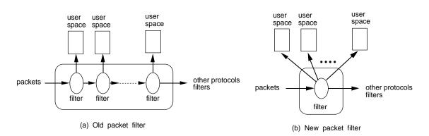
Figure 2: Redundant (BPF and CSPF) vs. one-step filtering (MPF) for incoming packets
