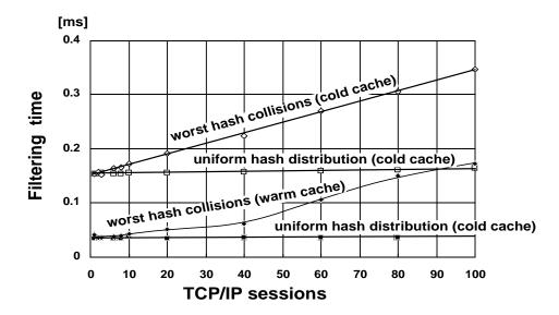
Figure 5: Effects of hash collisions. The curve from the previous experiment is shown for comparison.
