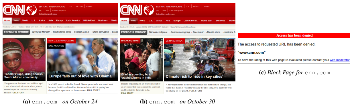
Figure 1: Differences between accessible pages inhibit block page detection. Figure 1a and Figure 1b are structurally similar, but contain different text and links. Both of these versions of the page differ from the block page in Figure 1c. The block page in Figure 1c also shows that block pages can contain custom content, in this case, the blocked URL, cnn.com . Variations in block page content make block page detection challenging and time consuming.
