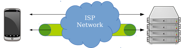
Figure 1: Schematic view of how our project works. Traffic is sent unencrypted and through the Meddle VPN tunnel between the mobile client and a control server.
