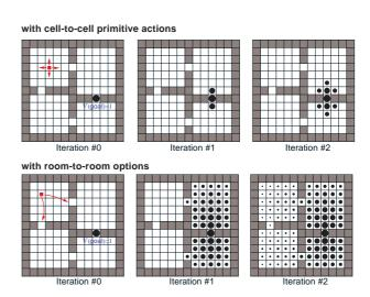
Figure 3: Value functions formed over iterations of planning by synchronous value iteration with primitive actions and with hallway options. The hallway options enable planning to proceed room-by-room rather than cell-by-cell. The area of the disk in each cell is proportional to the estimated value of the state, where a disk that just fills a cell represents a value of 1.0. We use discounting with  $\gamma=1$  for this task.
