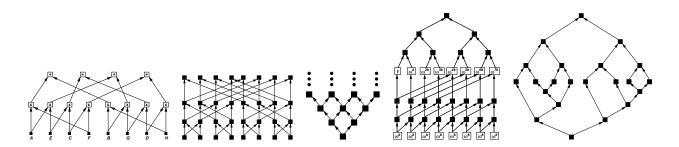
**Figure 1.** Data-dependency dags for (left to right): matrix multiplication, the Fast Fourier Transform (FFT), a generic wavefront computation, the discrete Laplace transform, a generic divide-and-conquer computation.
