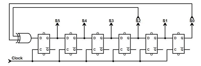
After each clock cycle, the output values for S0 through S4 will become the previous values from S1 through S5 (i.e., S5 is copied to S4 at the same time that S4 is copied to S3, S3 to S2, and so on). The new value in S5 will become the XOR of the old values of bits S2 and S0, but the old value of S0 is then lost.
