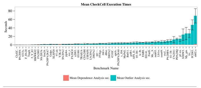
**Figure 10.** Mean CHECKCELL execution times. For most of the spreadsheets, CHECKCELL completes its analysis in under 30 seconds; for all but two, it completes in under 70 seconds (see Section 4.2). Error bars represent one standard deviation.
